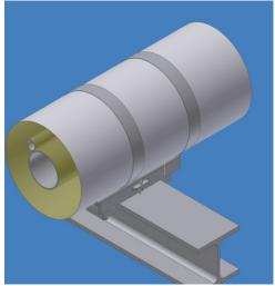
Picture 1 Isometric drawing of fix point support With insulation cover diam. 224mm
